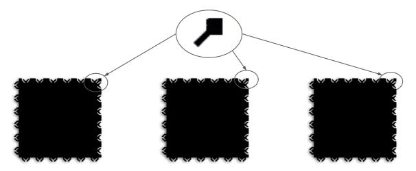
4) Use a normal cutter to finish the tiles along the walls, taking care to leave the sufficient space for thermal expansion.
